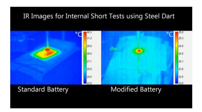
Researchers in the United States have modified the design of lithium-ion batteries to include slits along the electrodes, a feature which may mitigate the risk of battery failure during automobile accidents. The prototype, presented December 13 in the journal *Joule*, could allow manufacturers to scale down the housing materials that commonly protect batteries in electric cars from mechanical damage, improving the overall energy density and cost.
