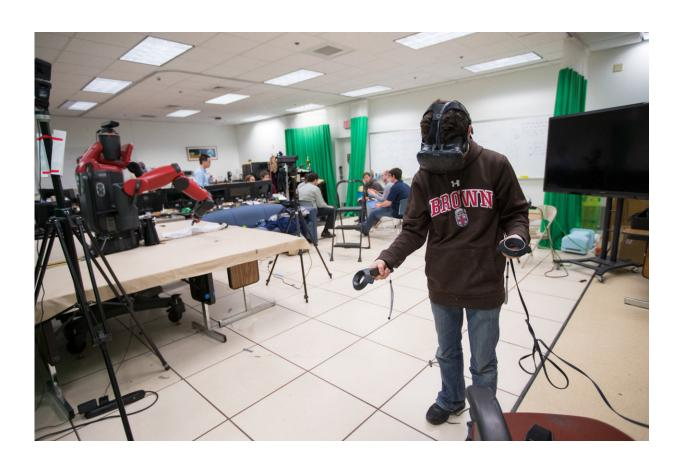
Brown University undergraduate Eric Rosen operates a Baxter robot using a virtual reality interface developed in Brown's Humans to Robots lab. Credit: Nick Dentamaro / Brown University
