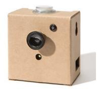
So with the kit, a Raspberry Pi Zero W and its camera become a neural network vision system.
