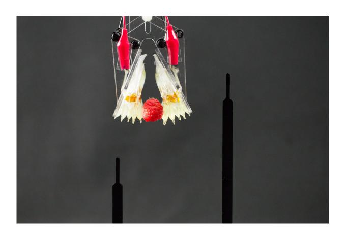
HASEL actuators can be designed as soft grippers to handle and manipulate delicate objects. Credit: Keplinger Lab / University of Colorado Boulder
