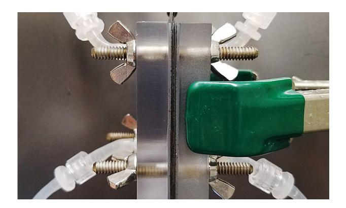
A feed solution contained in a reservoir was separately fed to the two inlets of the flow cell using pumps, one desalinated and the other concentrated. This is achieved by applying electrical current to the flow cell through wires using a power source (not shown in this photo). The conductivity of the discharge was then measured using flow conductivity meters located at each outlet, which were monitored by computer. Credit: Taeyoung Kim
