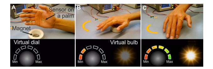
A skin-attached 2D magnetic field sensor allows the wearer to control the light intensity of a virtual bulb by rotating his hand over a magnetic field source. Credit: Helmholtz-Zentrum Dresden-Rossendorf e.V.
