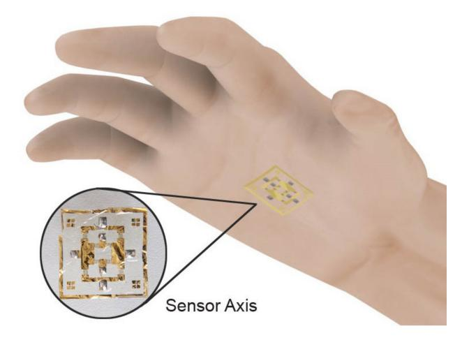
Schematics revealing a 2D magnetic field sensor mounted on a palm. Credit: Helmholtz-Zentrum Dresden-Rossendorf e.V.
