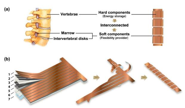
1-Copper current collectors, 2-Graphite anode, 3/6-Separator, 4-Lithium cobaltate cathode, 5-Aluminum current collectors, 7-Polyethylene supporting film.
