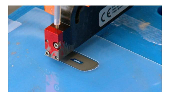
With a custom-built inkjet printer, Purdue researchers can deposit nanothermite with micron precision. Credit: Purdue University photo/Jared Pike
