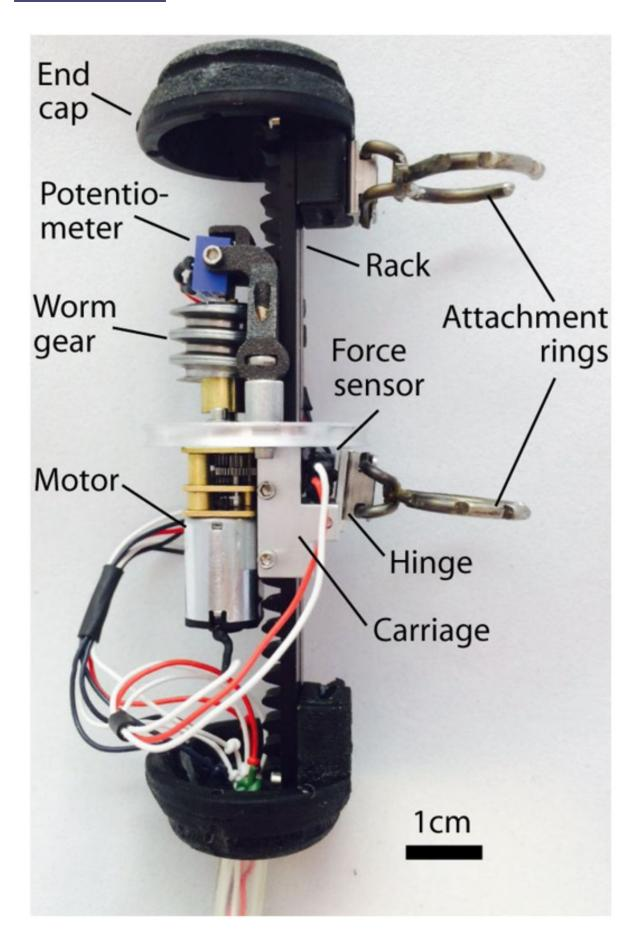
The esophagus-growing robotic implant. Credit: Damian et al., *Sci. Robot.* 3, eaaq0018 (2018)
