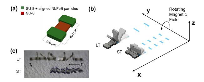
At left is a schematic of the new microTUM robot developed by researchers at Purdue University. The tiny robot tumbles in two modes, as shown at right. At bottom, a still photo of the microbot's motion is captured from a video. Credit: Purdue University image/ Chenghao Bi, Maria Guix
