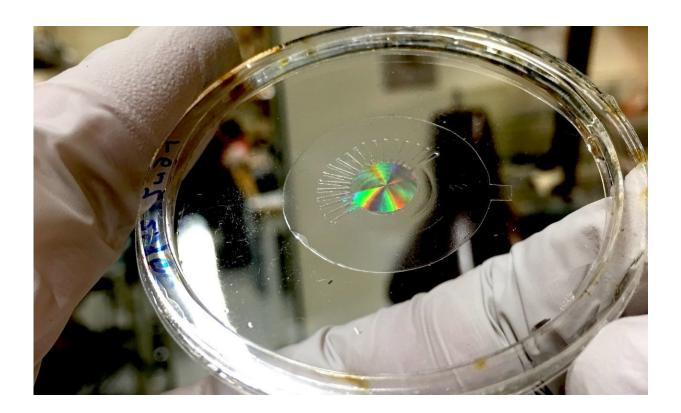
Photo of the metalens (made of silicon) mounted on a transparent, stretchy polymer film, without any electrodes. The colorful iridescence is produced by the large number of nanostructures within the metalens. Credit: Harvard SEAS
