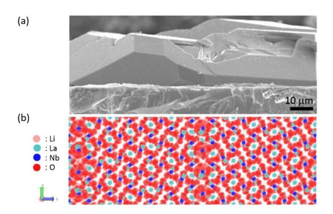
Image (a) is a cross-sectional SEM image of the Li5La3Nb2O12 crystal layer and image (b) shows computationally simulated trajectories of the Li, La, Nb, and O framework atoms obtained for  $\Sigma 3$  (2-1-1) = (1-21) at a temperature of 1300 K. Credit: Nobuyuki Zettsu Ph.D., the Center for Energy and Environmental Science, the Department of Materials Chemistry, Shinshu University.
