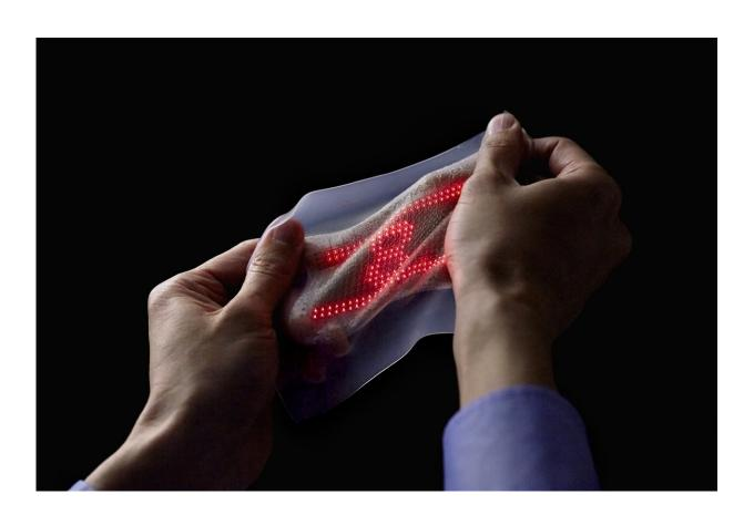
The soft, flexible skin display is about 1 millimeter thick, and consists of a 16 x 24 array of micro LEDs and stretchable wiring mounted on a rubber sheet. It can withstand repeated stretching, by as much as 45 percent of its original length, without showing any loss in function of its electrical and mechanical properties. Credit: 2018 Takao Someya Research Group.
