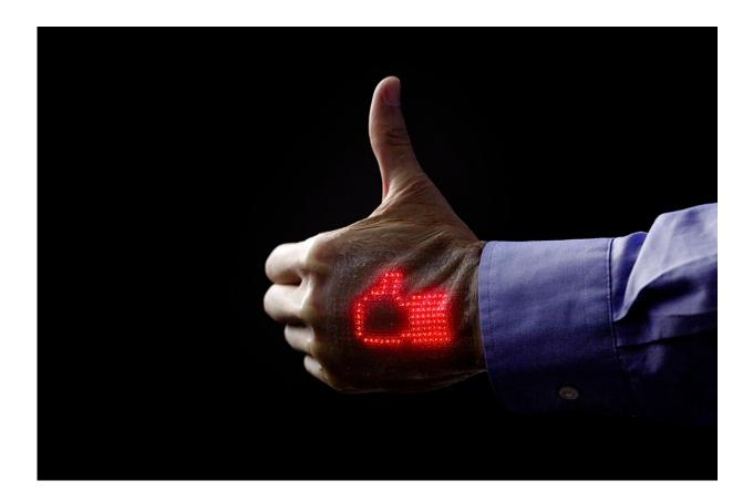
An integrated "skin electronics" system allows health monitoring at home and gives doctors remote access to biometric data transmitted wirelessly to a medical cloud. It promises to enhance self-care and accessibility of medical information to various segments of the population, including children and the elderly. A thumbs-up image on the skin display serves as an indicator of good health. Credit: 2018 Takao Someya Research Group.
