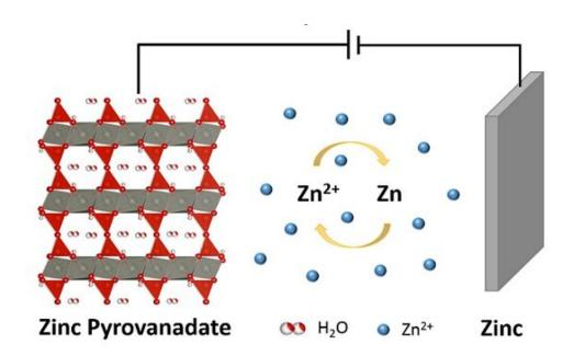
A simple method for creating zinc pyrovandate electrodes improves the performance of zinc-ion batteries. Credit: KAUST
