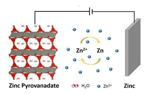
A simple method for creating zinc pyrovandate electrodes improves the performance of zinc-ion batteries. Credit: KAUST
