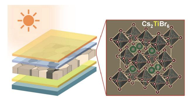
Researchers have shown that titanium is an attractive choice to replace the toxic lead in the prevailing perovskite thin film solar cells. Credit: Padture Lab / Brown University
