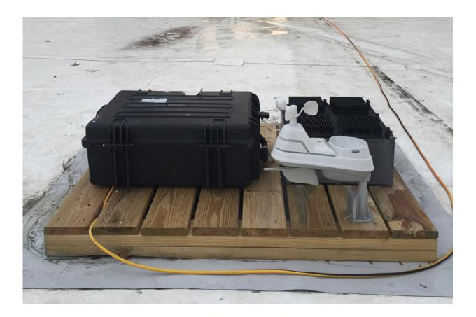
The team's test device, which has been deployed on the roof of an MIT building for several months, was used to prove the principle behind their new energyharvesting concept. The test device is the black box at right, behind a weathermonitoring system (white) and a set of test equipment to monitor the device's performance (larger black case at left). Credit: Justin Raymond
