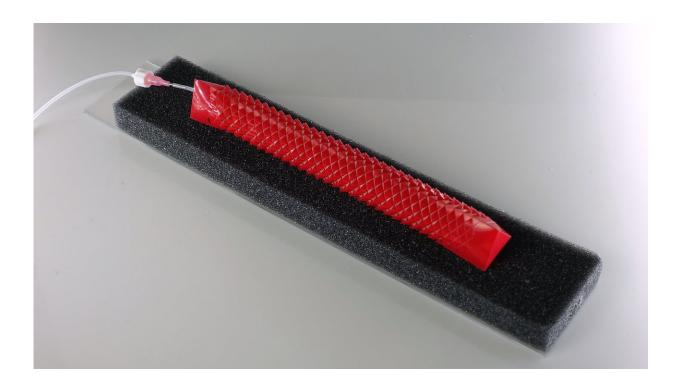
This soft robot is made using kirigami -- an ancient Japanese paper craft that relies on cuts, rather than origami folds, to change the properties of a material. As the robot stretches, the kirigami is transformed into a 3-D-textured surface, which grips the ground just like snakeskin. Credit: Ahmad Rafsanjani/Harvard SEAS
