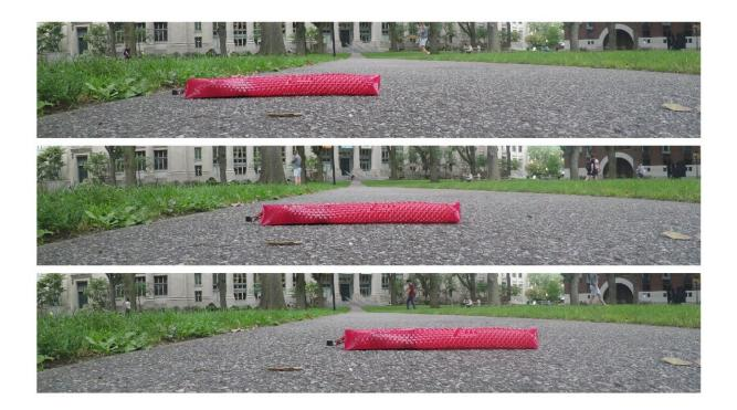
Harvard researchers built a fully untethered, bioinspired soft robot, with integrated onboard control, sensing, actuation and power supply packed into a tiny tail. Credit: Ahmad Rafsanjani/Harvard SEAS
