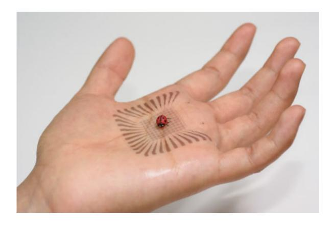
Pixelated electronics built with skin-like materials conform to the complex curves of a hand. Credit: L.A. Cicero
