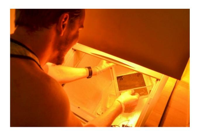
Karl Vitale positions a scale model of the Melt Mat, a type of thermal absorptive blanket, inside an experimental set up equipped with artificial sunlight that allowed students to monitor the rate of snow melt over time. Vitale belonged to an undergraduate senior project team in the Department of Biomedical Engineering and Mechanics that designed, constructed, and tested the Melt Mat, which accelerates snow melting times by threefold. Credit: Virginia Tech
