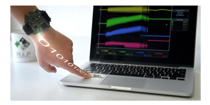
A multi-sensor wristband that uses touch communication to transmit signals through the human body to a zero-power receiver on a laptop computer. Credit: Michele Magno / ETH Zurich
