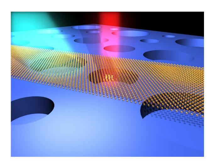
Illustration of ultrasensitive optical interrogation of the motions of atomically thin drumhead nanoelectromechanical resonators (made of atomic layers of MoS2 semiconductor crystals). Credit: Case Western Reserve University
