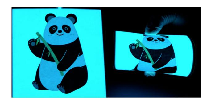
Pieces of flexible, rechargeable yarn batteries can be connected in series to power electroluminescent panel displays. Credit: American Chemical Society
