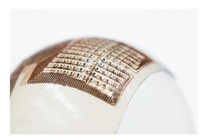
This stretchable, flexible ultrasound patch could make it easier to inspect damage deep inside odd-shaped structures, such as engine parts, turbines, reactor pipe elbows and railroad tracks--objects that are difficult to examine using conventional ultrasound equipment. Credit: Hongjie Hu
