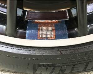
This stretchable, flexible ultrasound patch can easily conform to odd-shaped surfaces such as pipe elbows (left) and wheel edges (right)--objects that are difficult to probe with conventional ultrasound equipment. Credit: Hongjie Hu
