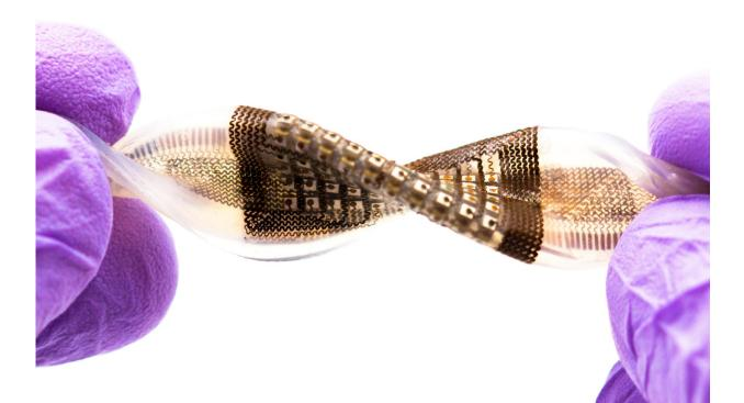
This stretchable, flexible ultrasound patch could make it easier to inspect damage deep inside odd-shaped structures, such as engine parts, turbines, reactor pipe elbows and railroad tracks--objects that are difficult to examine using conventional ultrasound equipment. Credit: Hongjie Hu
