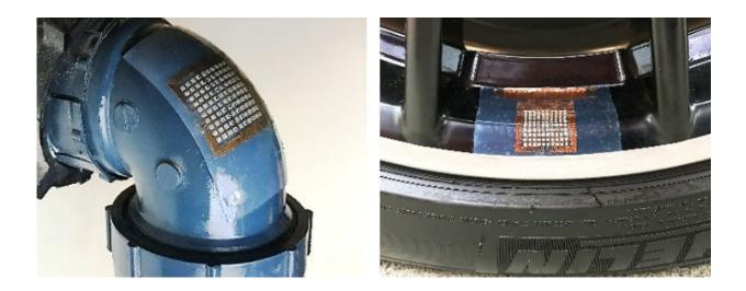
This stretchable, flexible ultrasound patch can easily conform to odd-shaped surfaces such as pipe elbows (left) and wheel edges (right)--objects that are difficult to probe with conventional ultrasound equipment. Credit: Hongjie Hu
