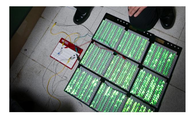
Georgia Tech professor Zhong Lin Wang poses with an array of 1,000 LED lights that can be illuminated by power produced by the force of a shoe striking a triboelectric generator placed on the floor. Credit: Rob Felt
