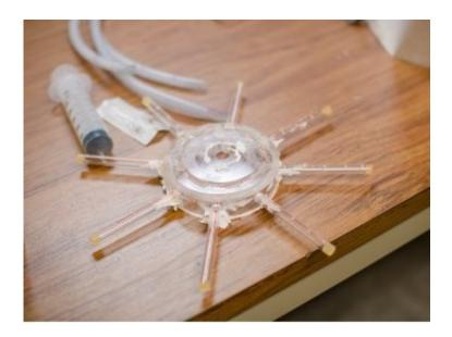
The PVC spraying mechanism that causes the water to circulate constantly within a tank to prevent a stagnant top layer clotted with algae and bacteria. Credit: Michigan Technological University
