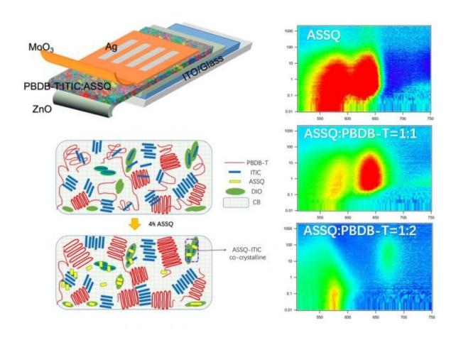
The research team led by André Taylor, working with the active layer of an organic solar cell, achieved remarkable efficiency by introducing a squarine molecule (ASSQ) as a crystallizing agent, which both donates electrons and enhances the light absorption of the active layer of the cell, properly orienting the PBDB-T donor-acceptor polymer that accepts the donor electron with the with the non-fullerene electron-acceptor molecule ITIC. Credit: NYU Tandon
