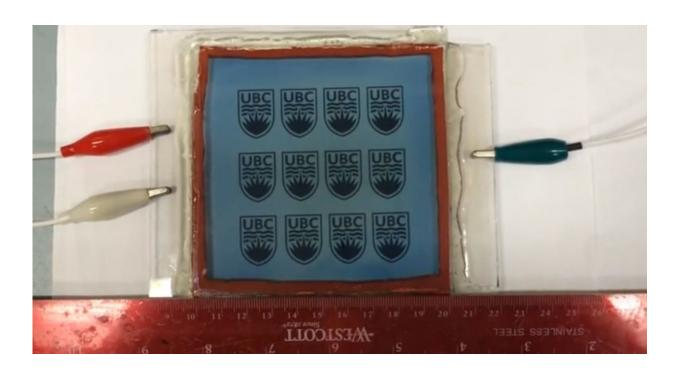
UBC chemistry researchers have developed a simple, cost-effective technique for making smart windows that could lead the way for wide-scale adoption of this energy-saving technology.
