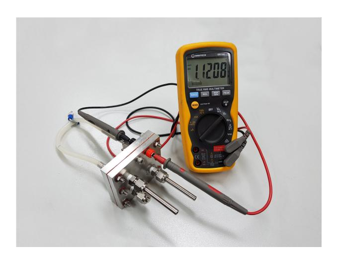
The RMIT-developed proton battery connected to a voltmeter. The working prototype has an energy per unit mass already comparable with commercially-available lithium ion batteries. Credit: RMIT University
