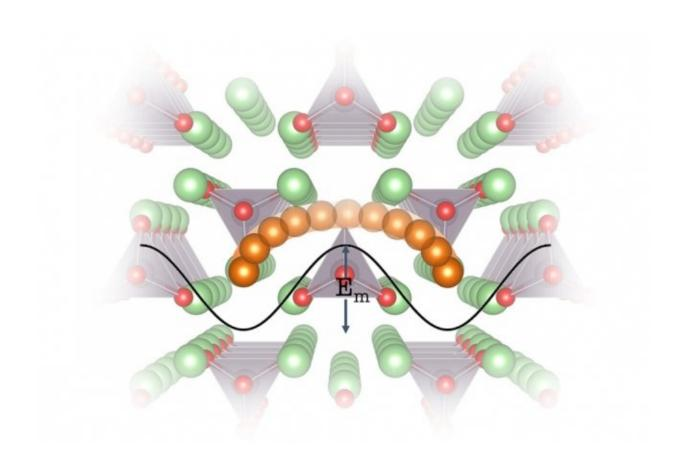
Diagram illustrates the crystal lattice of a proposed battery electrolyte material called Li3PO4. The researchers found that measuring how vibrations of sound move through the lattice could reveal how well ions – electrically charged atoms or molecules – could travel through the solid material, and therefore how they would work in a real battery. In this diagram, the oxygen atoms are shown in red, the purple pyramid-like shapes are phosphate (PO4) molecules. The orange and
