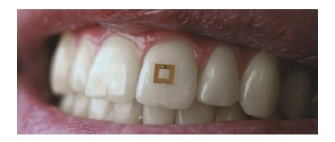
The 2x2 mm sensor monitors ingested fluids and transmits information wirelessly. Credit: Fio Omenetto, Ph.D., Tufts University
