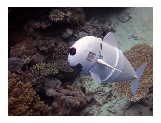
Using its undulating tail and a unique ability to control its own buoyancy, SoFi can swim in a straight line, turn, or dive up or down. Credit: MIT CSAIL
