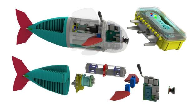
SoFi's lightweight setup includes a single camera, a motor, and the same lithium polymer battery that can be found in consumer smartphones. Credit:
