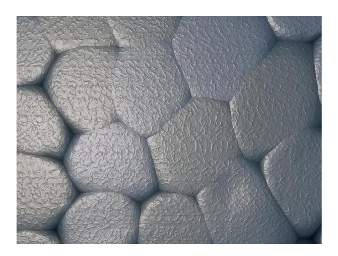
Image shows the temperature driven merging and fusing of lithium dendrites into a uniform (smooth) surface, which eliminates the risk of electrical shorting in lithium-ion batteries. Credit: Rensselaer Polytechnic Institute
