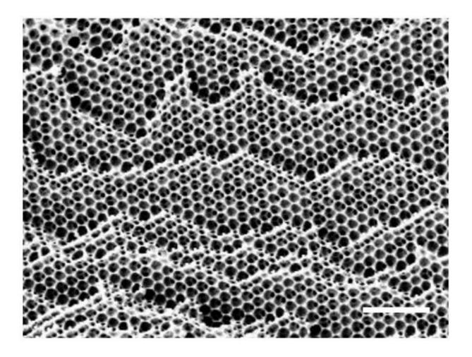
Magnification of the cross section of the microgroove-patterned color-changing hydrogel. Credit: Fu et al., *Sci. Robot.* 3, eaar8580 (2018)
