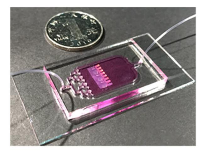
The biohybrid structural color-changing hydrogel integrated on a heart-on-achip. Credit: Fu et al., *Sci. Robot.* 3, eaar8580 (2018)
