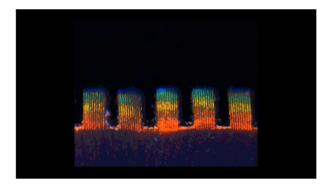
To demonstrate the effectiveness of the heart-on-a-chip system made of the color-changing biohybrid hydrogel, various concentrations of the drug isoproterenol were pumped into the chip to stimulate the heart cells. This close-up of the chip shows the color shift to blue when isoproterenol was added. Credit: Fu et al., *Sci. Robot.* 3, eaar8580 (2018)
