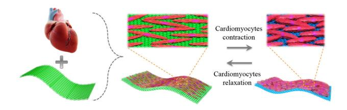
Schematic diagram of the construction of the bioinspired self-regulated structural color hydrogels by assembling engineered cardiomyocyte tissues on synthetic inverse opal hydrogel films. Credit: Fu et al., *Sci. Robot.* 3, eaar8580 (2018)
