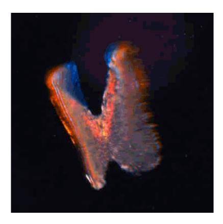
The 3-D robotic butterfly made from the color-changing biohybrid hydrogel. Credit: Fu et al., *Sci. Robot.* 3, eaar8580 (2018)
