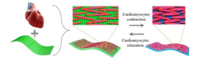
Schematic diagram of the construction of the bioinspired self-regulated structural color hydrogels by assembling engineered cardiomyocyte tissues on synthetic inverse opal hydrogel films. Credit: Fu et al., *Sci. Robot.* 3, eaar8580 (2018)
