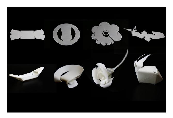
A computer-controlled process developed at Carnegie Mellon University enables flat pieces of plastic produced in an inexpensive 3-D printer to assume predetermined 3-D shapes when heated. Credit: Carnegie Mellon University
