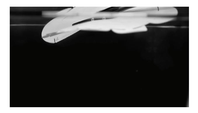
A process developed at Carnegie Mellon University enables a flat piece of plastic produced in an inexpensive 3-D printer to assume the shape of a rose when dipped in hot water. Credit: Carnegie Mellon University
