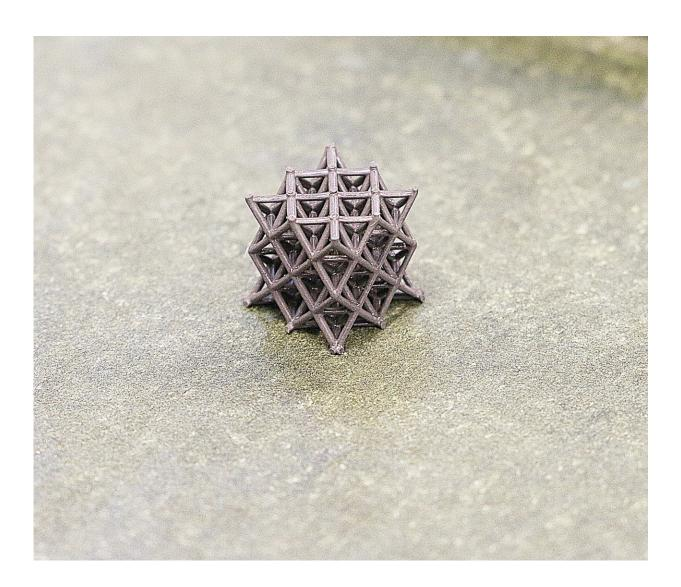
Sample of the 3-D printed acoustic metamaterial. Credit: Qiming Wang
