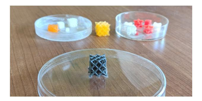
The magnetoactive acoustic metamaterial (center front) affixed to a petri dish.
