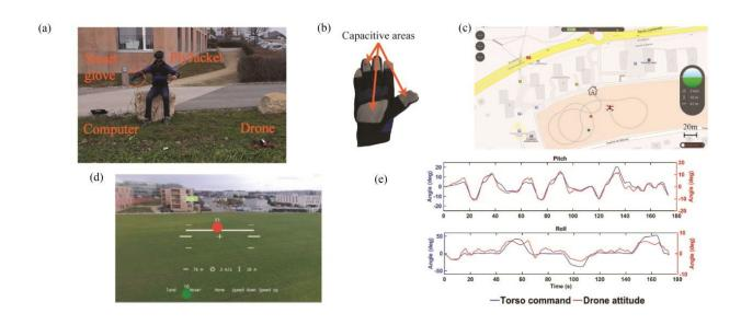
Real teleoperation of a drone. (a) User and setup. (b) Smart glove with capacitive sensors. (c) Map and drone route. (d) View from the head mounted display. (e) Logs of the flight. Credit: *IEEE Robotics and Automation Letters* (2018). DOI: 10.1109/LRA.2018.2810955
