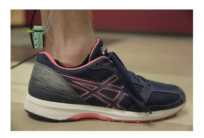
UW-Madison researchers developed a simple, noninvasive wearable device that enables them to measure tendon tension while a person is engaging in activities like walking or running. Here, the device is placed over the Achilles tendon. Credit: Renee Meiller/UW-Madison
