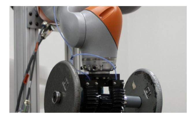
Researchers mounted a slightly modified version of the gripper on a robotic arm at JPL. They showed it's capable of lifting up to 45 lbs. Credit: JPL
