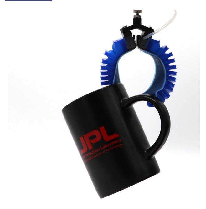
The gripper can easily manipulate objects like mugs. Credit: University of California San Diego and JPL
