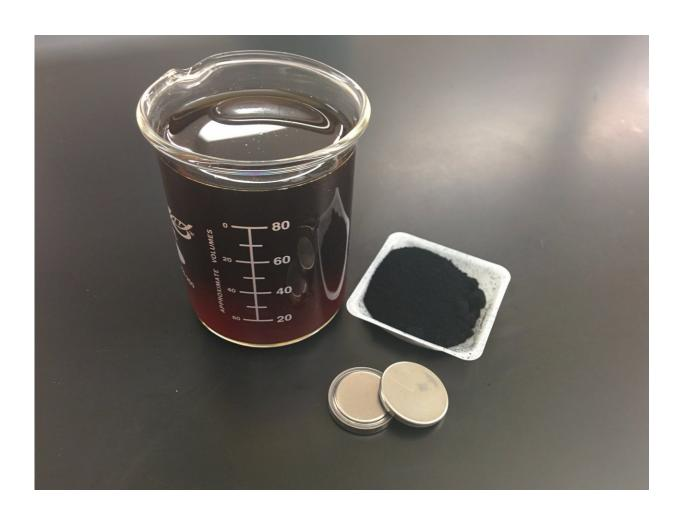
Researchers at Rensselaer Polytechnic Institute have developed a patented method to use cheap and abundant paper biomass to make lithium-sulfur batteries. Credit: Rensselaer Polytechnic Institute
