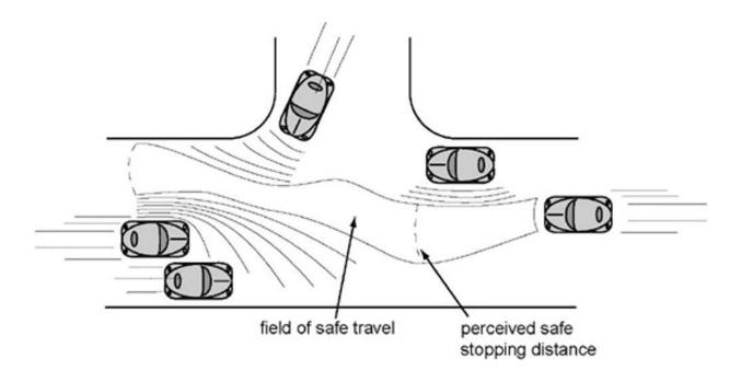
The driver of the car on the right judges a safe path through obstacles based on their movements and perceived stopping distances. Credit: Adapted from Gibson and Crooks by Steven Lehar
