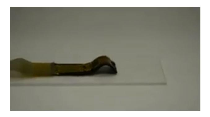
If Star Wars' R2-D2 is your idea of a robot, think again. Researchers led by a University of Houston engineer have reported a new class of soft robot, composed of ultrathin sensing, actuating electronics and temperature-sensitive artificial muscle that can adapt to the environment and crawl, similar to the movement of an inchworm or caterpillar.
