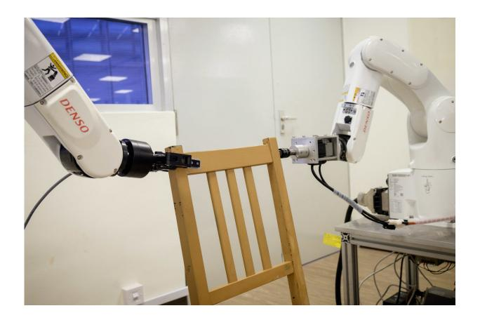
The NTU robot is designed to mimic the genericity of human "hardware" used to assemble objects. For instance, each robotic arm is equipped with parallel grippers to pick up objects, and has force sensors to determine how strongly the "fingers" are gripping. This makes the robot more human-like in its manipulation of objects. Credit: NTU Singapore
