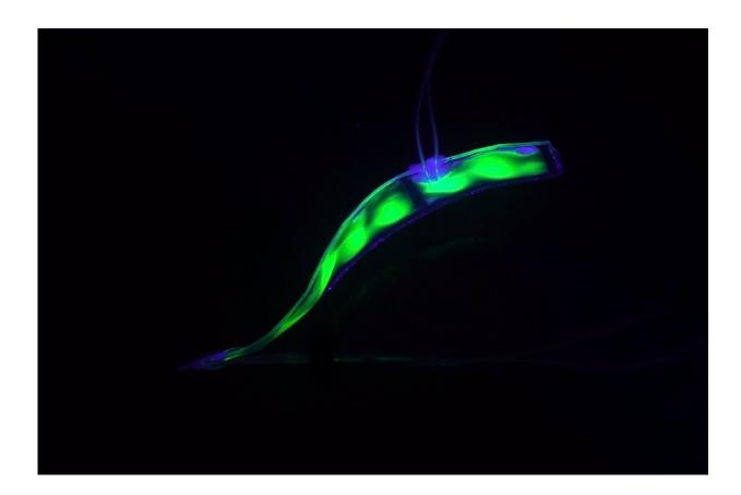
The conductive chambers inside the robot's artificial muscles can be loaded with fluorescent dye (as shown in the video accompanying the study and this release). In the future, the fluorescence could be used as a kind of signaling system. Credit: University of California San Diego
