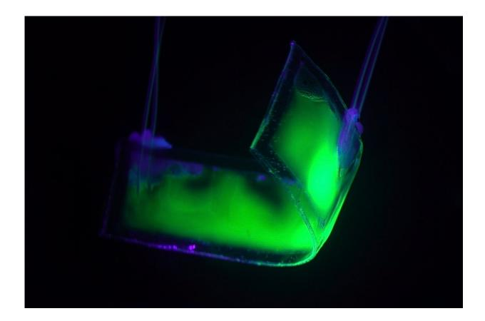
Instead of propellers, our robot uses soft artificial muscles to move like an eel underwater without making any sound. Credit: University of California San Diego
