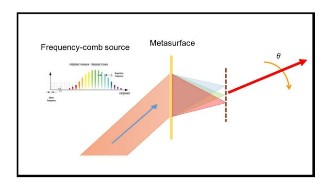
A novel laser light sensing technology would use an optical metasurface and an input ultrafast pulse with a spectrum that consists of frequency comb, or equally spaced phase-locked frequency lines. The metasurface focuses these frequency components to an array of adjacent locations in space. These focused locations
