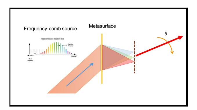
A novel laser light sensing technology would use an optical metasurface and an input ultrafast pulse with a spectrum that consists of frequency comb, or equally spaced phase-locked frequency lines. The metasurface focuses these frequency components to an array of adjacent locations in space. These focused locations
