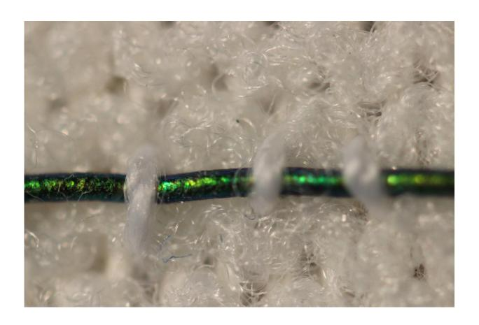
Engineers at MIT have developed pressure-sensing photonic fibers that they have woven into a typical compression bandage. Credit: Massachusetts Institute of Technology
