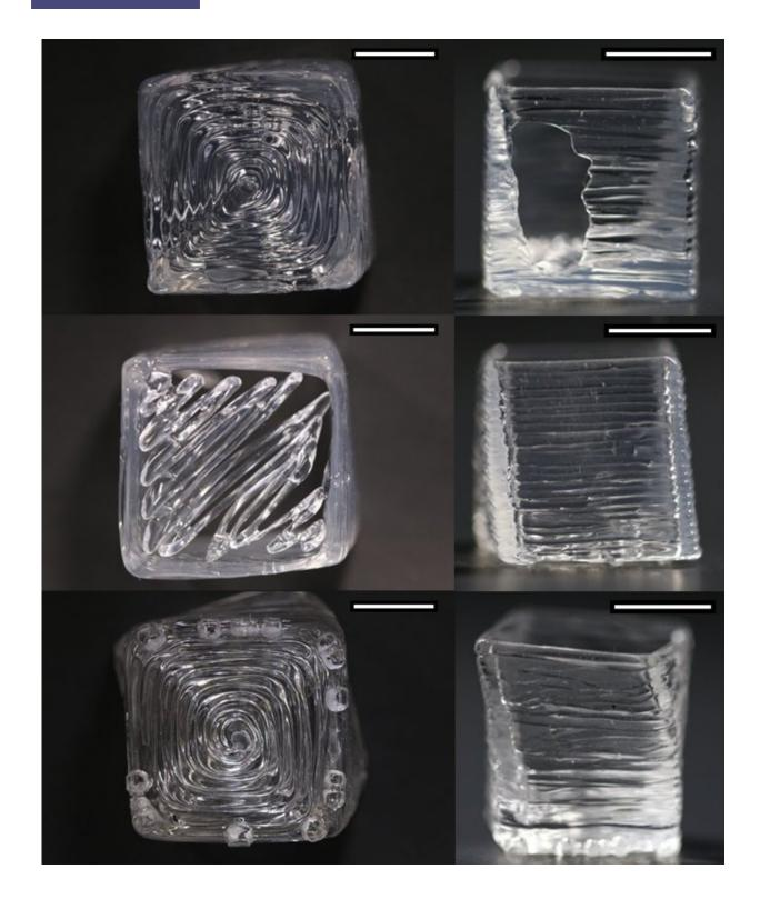
Images of the PDMS 3D prints made using the S3D CAD slicer to determine toolpath. Credit: Sara Abdollahi, Alexander Davis, John H. Miller, Adam W. Feinberg
