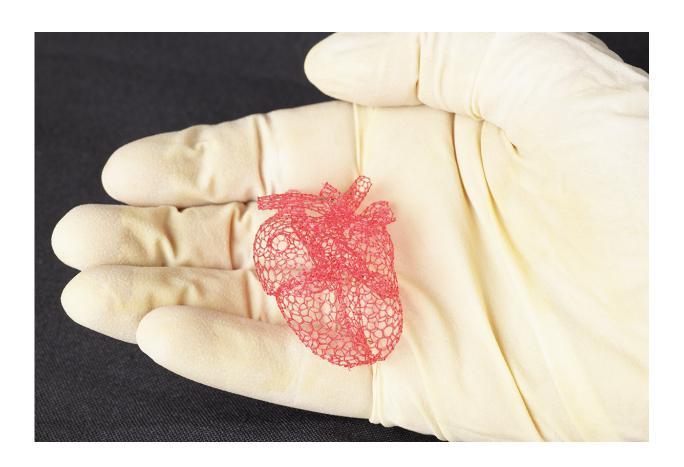
Freeform printing allows the researchers to make intricate structures, such as this model of a heart, that could not be made with traditional layer-by-layer 3-D printing. The structures could be used as scaffolds for tissue engineering or device manufacturing. Credit: Travis Ross, Beckman Institute
