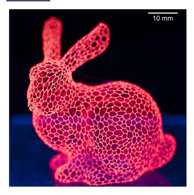
A 3-D printed bunny made of isomalt sugar mixed with a glowing red dye used in biomedical imaging. Credit: Troy Comi
