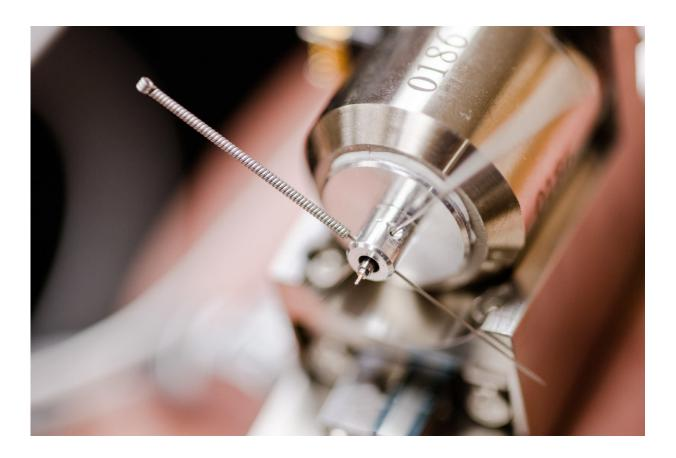
The diamond-tipped probe Herbert and Hackney use for their research is incredibly sensitive and must be housed in a compartment that muffles any sort of vibrations. Credit: Sarah Bird/Michigan Tech
