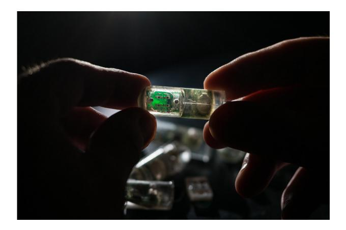
MIT engineers have designed an ingestible sensor with bacteria programmed to sense environmental conditions and relay the information to an electronic circuit. Credit: Lillie Paquette, MIT
