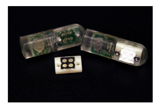
Bacteria engineered to detect specific molecules are placed in four wells on the custom-designed sensor, which is attached to a microprocessor that converts the sensory information to a wireless signal. Credit: Melanie Gonick, MIT
