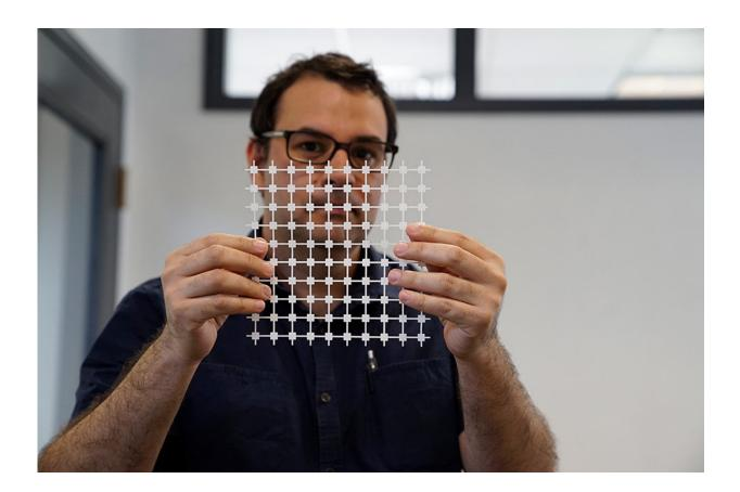
Jose Gomez-Marquez, co-director of MIT's Little Devices Lab, holds a sheet of paper diagnostic blocks, which can be easily printed and then combined in various ways to create customized diagnostic devices. Credit: Melanie Gonick/MIT
